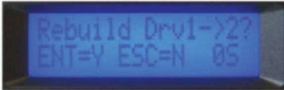
5. Push the ENT button to begin the process or ESC button to cancel. Alternately, the process will automatically cancel in 10 seconds.
