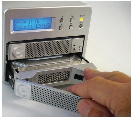
4. G-SAFE will ask if you would like to rebuild the array. In our example, G-SAFE will rebuild from Drive 1 (top drive) to Drive 2 (bottom drive).
