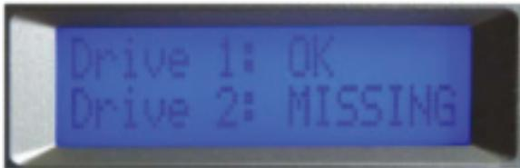
**Drive Failure:** If a drive failure occurs, the LCD will indicate which disk must be replaced. See [Replacing a Disk Drive Module](#) for how to do this.
