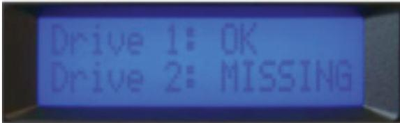
2. Turn on G-SAFE. The alarm will sound and the display will indicate a MISSING drive. Mute the alarm by pressing the Mute button on the front panel.
