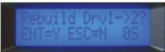
6. Push the ENT button to begin the process or ESC button to cancel. Alternately, the process will automatically cancel in 10 seconds.
