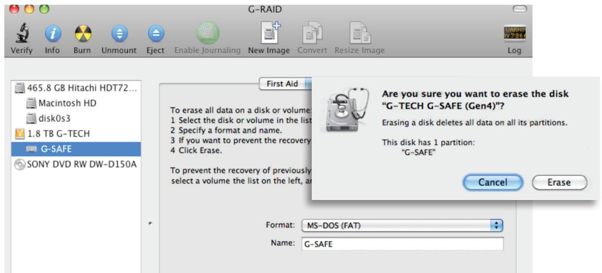
5. Click the Erase button. A progress bar in the lower right corner of the window will show the progress of the disk's reformatting. Your drive will be formatted to its full capacity as FAT32.
