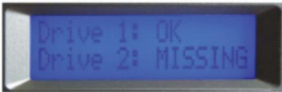
4. Insert one of the original (compromised) drive modules in the open bay. **WARNING:** The target drive you are inserting will be overwritten with data from the source drive. Be sure you are inserting the correct drive.
