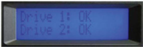
All data saved to G-SAFE is simultaneously written (mirrored) to the system's two removable disk drive modules providing an instant back up of your data. If one of the disk drive modules in G-SAFE should fail, your data is safe and accessible.
